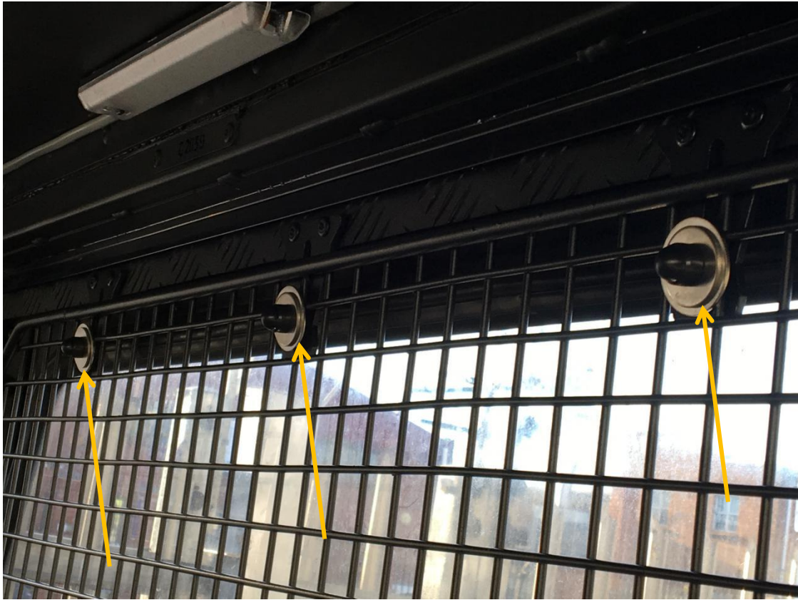
Figure 10: Spaced out Top Vertical Mounts installed
